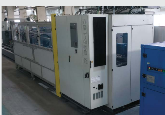
Stator Injection Machine Injection Length - Up to 8000 mm
