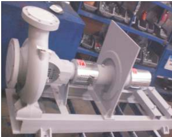
Seawater Cooling Pump - 4000 DWT Oil Tanker with Bulkhead Penetration, Bashundhara Steel & Engineering Ltd., Bangladesh
